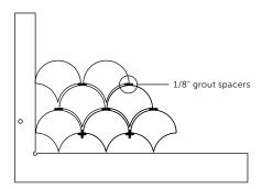
Use 1/8" grout spacers and continue laying the tiles. The 1/8" spacers end up making the grout joint about 3/16" due to the tile's cushion edge.
