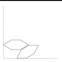
The easiest way to start the Braided Pattern for a kitchen backsplash is to orient the tile horizontally, stair stepping up and to the right.
