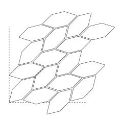
Continue adding pieces until your area is filled. Make cuts using a tile wet saw.
