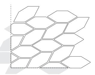
Lay tile in the open spaces of the tiled area and use a pencil and straight edge to mark the cuts. Use the lines drawn on the paper as a guide. Cut the tile using a tile wet saw.
