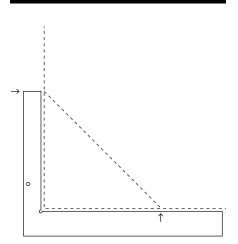
To begin the vertical layout, draw a line connecting your square line from the same measurement point on each side. For example, find 10" on both edges of your square and draw a line between those points.
