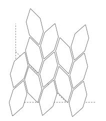
Continue adding pieces until your area is filled. Make cuts using a tile wet saw.
